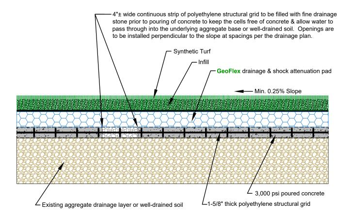
Detail #2 ~ Turf Installation over Opening in Concrete for Drainage
