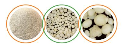
GeoCool has a specific gravity similar to sports field sand which means it will not float in heavy rain events and will not blow away in dry, windy environments.
